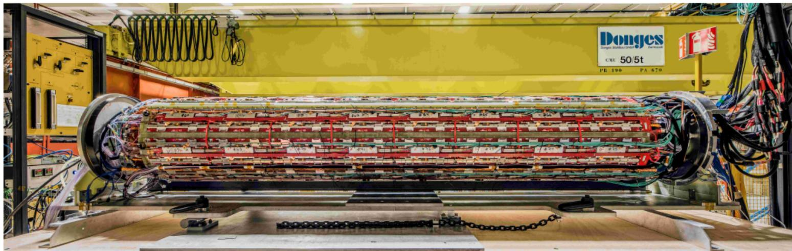
Gas detector to track charged particles produced by  $\bar{H}$  annihilation.
